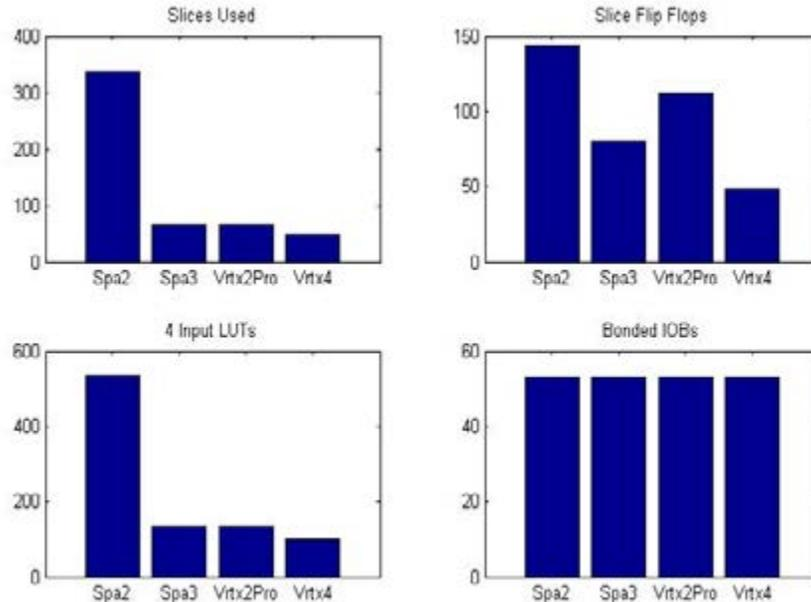
Figure 8 : Resource utilization in different target platforms. (Where Spa2= Spartan2 xc2s200-6fg456, Spa3= Spartan3E xc3s500e -5fg320, Vrtx2Pro = Virtex2Pro xc2vp30 ff6896, Vrtx4= Virtex4 xc4vfx12 ML402, LUTs = Look up tables, IOBs = Input or output blocks)
