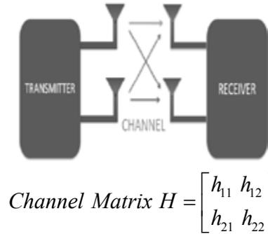
$$ST \text{ Block Code Input } X_t = \begin{bmatrix} s_1 & s_2 \\ -s_2^* & s_1^* \end{bmatrix}$$
